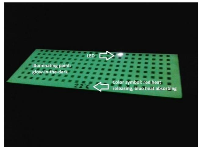
Picture 4: artificial light is being switched off. The glow-in-the-dark paint and the LED is now illuminating the room.
