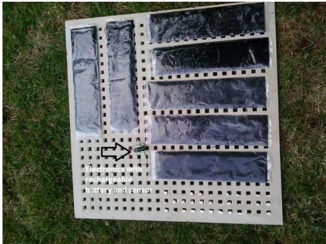
Picture 1: rear side with PCM bags. At this side also the sensor and the battery is constructed
