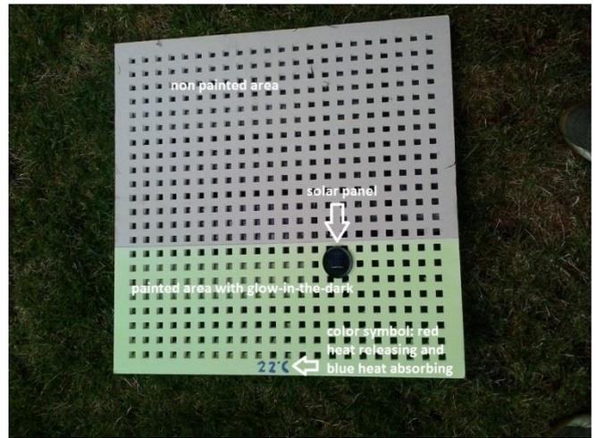
Picture 2: tile painted for 30% with light glow-in-the-dark (green). At this side the solar panel is visible.
